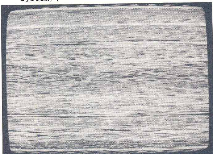
A picture scrambled by active line rotation a possible system for future subscription services (see page 3).
