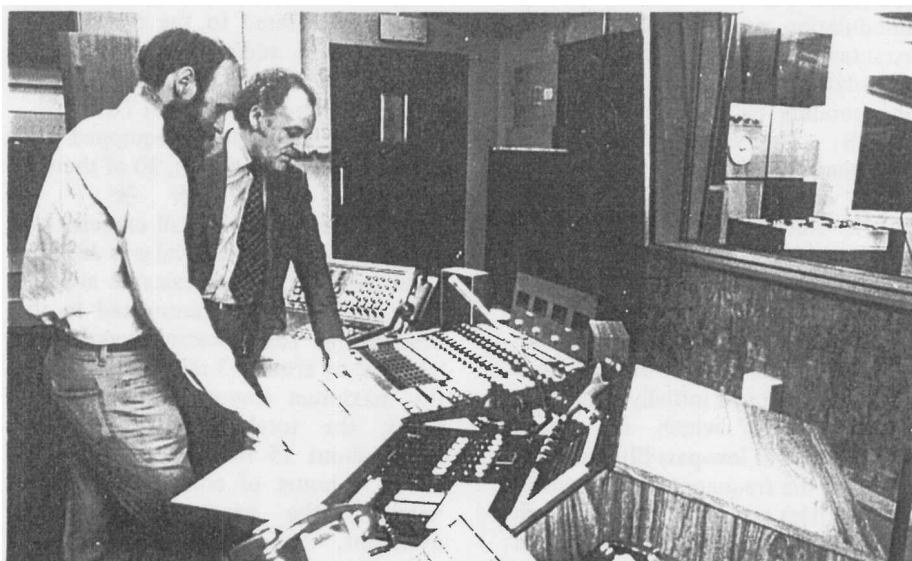
Jimmy Jewel! (right), of SCPD, discusses the Neve 12-channel, 2-output sound desk with Peter Rowe, an engineer in Communications Engineering Services at Glasgow, in the new production continuity control cubicle. The studio can be seen through the window on the right.
