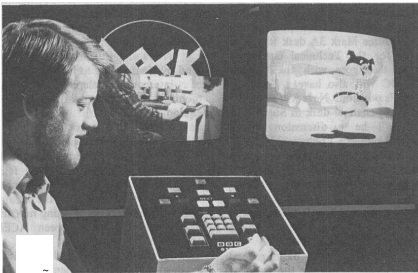
Adrián Durey, Research Department, operates the control keyboard of the prototype studio store. A new picture has just been accessed and is being output via the preview output. The main output is displayed on the right-hand monitor.
