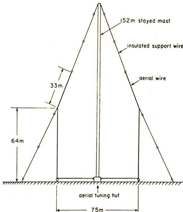
**Figure 2. 1149 kHz/1214 kHz antenna suspended from a 500-foot mast at Moorside Edge**
