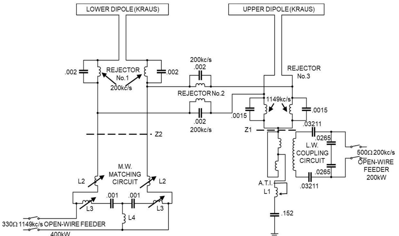
Figure 1. HPMW and 5GB (LF) Antenna Tuning House circuits for combining and matching
