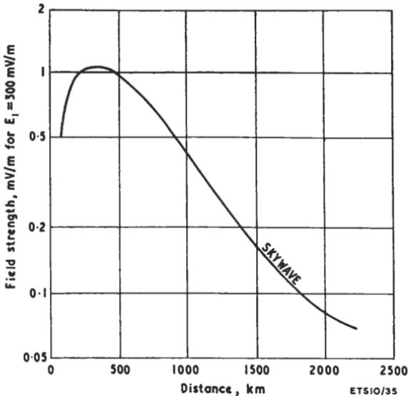
Fig. 24. Quasi-maximum field strength of sky wave at night; the field strengths shown are those exceeded instantaneously for five per cent of the time
