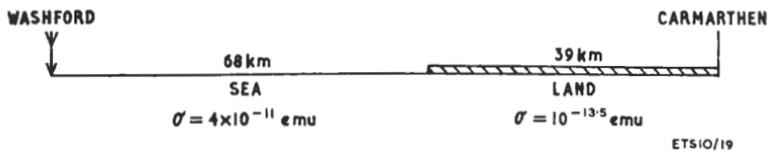
Fig. 12. Mixed-path propagation example. Washford to Carmarthen
