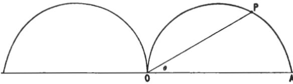
Fig. 1. Vertical radiation pattern for short aerial
