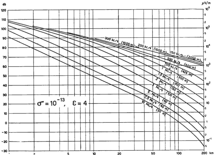
Fig. 7. Propagation over land of good conductivity (conductivity  $\sigma = 10^{-13}$  e.m.u., dielectric constant  $\epsilon = 4$  e.s.u.)  $E_1 = 300$  mV/m
