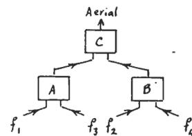
Fig. 31. Method of combining four u.h.f. channels.
