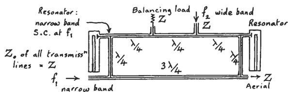
any frequencies other than  $f_1$ , which enter the  $f_1$  port and also absorbs any frequencies which enter the  $f_2$  port and manage to get past the resonators. The length of the ring should be electrically two-wavelengths at the  $f_1$  frequency in order to obtain maximum cross-loss at that frequency.
