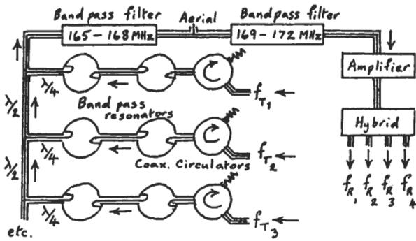
Fig. 39. Combiner using resonators and circulators.
