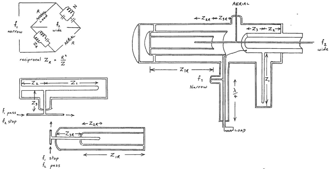
Fig. 41. Maxwell-bridge coaxial combiner.
