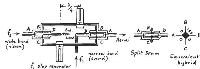
Fig. 29. U.h.f. combiner using hybrids and resonators.
