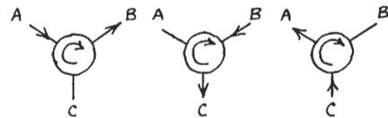
Fig. 17. Circulator power directions.
