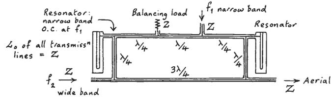
Fig. 23. Two-wavelength ring.
