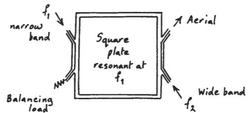
Fig. 35. Resonant plate combiner.
