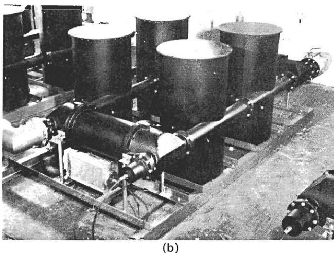
interconnecting transmission lines and use the back-to-back hybrid mode to reach the aerial. If the resonators do not appear as complete open-circuits, some power from the  $f_2$  transmitter will be reflected back into the balancing load instead of being transferred to the aerial. Power from the  $f_2$  transmitter is prevented from reaching the  $f_1$  transmitter only by the 'output balance' of the hybrids, which cannot be perfect at all frequencies in a system using 3 dB couplers.
