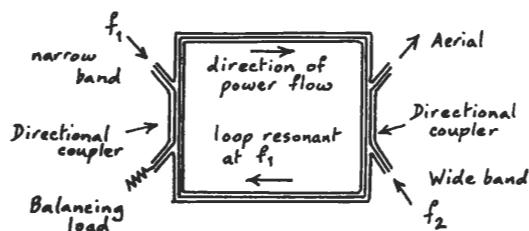
Fig. 34. Travelling-wave combiner.
