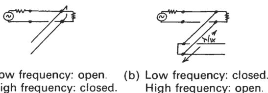
system this may be carried out by connecting a quarter-wave of low-loss feeder between the through-line and the tapping point on the stub as shown in Fig. 7. Intermediate lengths of connecting feeder can be used to vary the 'open' and 'closed' bandwidths.
