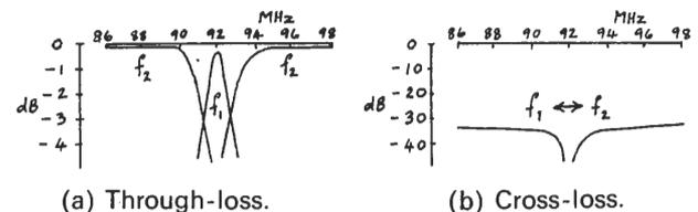
**Fig. 27.** Four-resonator v.h.f. combiner performance
