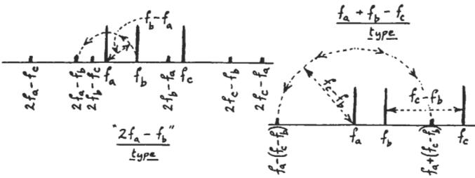
Fig. 9. Intermodulation frequencies.
