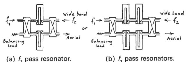
four-resonator v.h.f. combiner operating in this mode are shown in Fig. 27.
