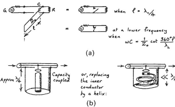
Fig. 5. Resonator 'frequency switch'.
