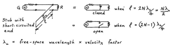
Fig. 4. Long-line 'frequency switch'.
