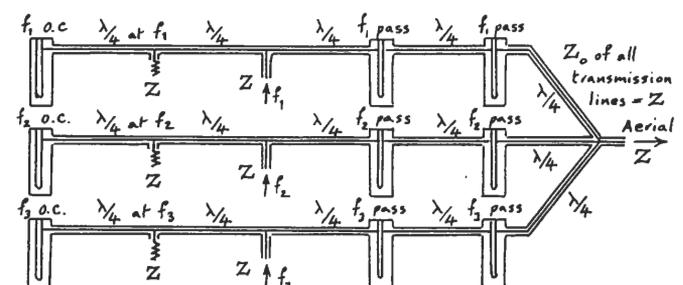
in each input chain present an open-circuit in shunt with the transmission line to which they are attached. The result of this is to open up the path to the aerial and to put an effective short-circuit across the balancing load at the input frequency. At other frequencies in the band the path to the aerial is closed and power from the transmitter is diverted to the balancing load. The characteristic impedance of all transmission lines is normally equal to the input and output impedances.
