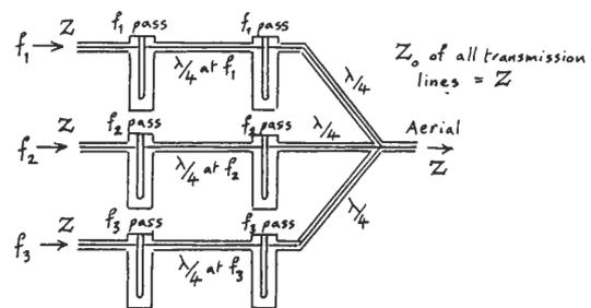
Fig. 21. Non-constant impedance parallel combiner using resonators.
