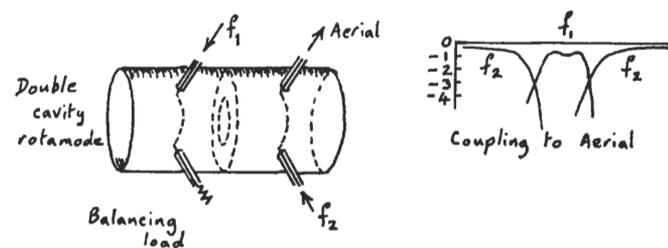
Fig. 38. Waveguide channel combiner.
