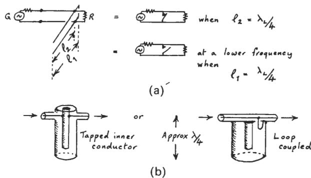
Fig. 6. Resonator 'frequency switch'.
