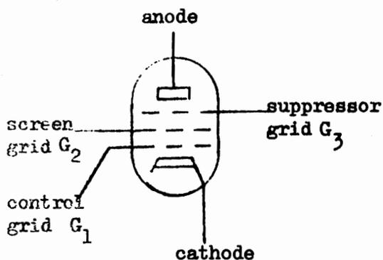
Fig. 11 : The Electrodes of a Pentode Valve
