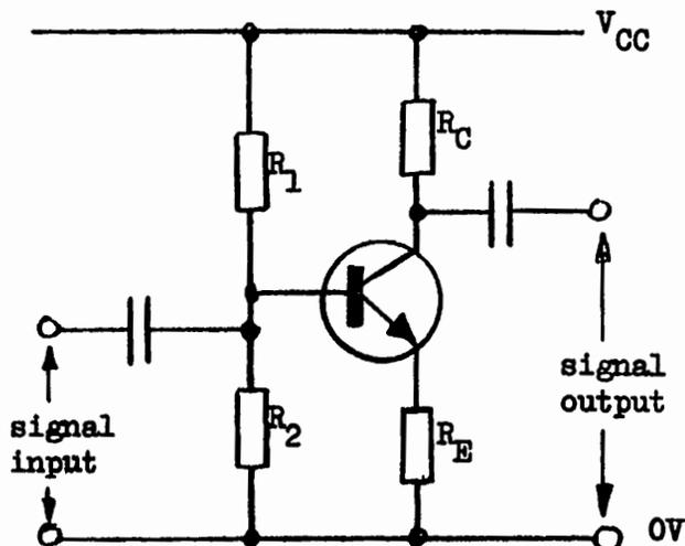
Fig. 2 : An improved transistor amplifier
