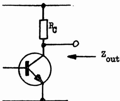
Fig. 4 : Output Impedance of Amplifier
