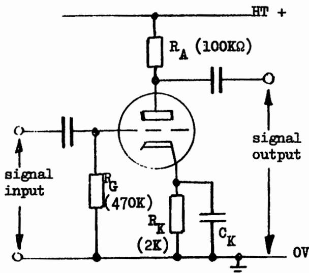
Fig. 8 : A Common Cathode Amplifier
