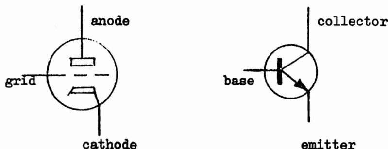
Fig. 7 : Similarity between electrodes of a valve and a transistor
