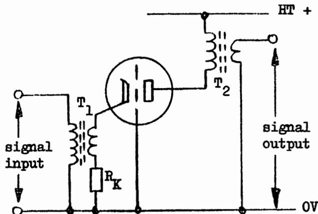
Fig. 9 : A Common Grid Amplifier for use at high radio frequencies
