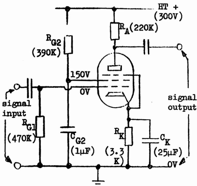
Fig. 12 : A Pentode used as an A.F. Amplifier
