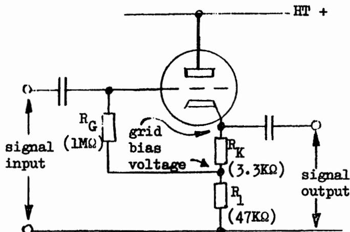
Fig. 10 : A Common Anode Amplifier
