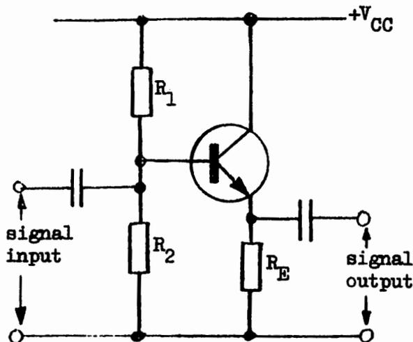
Fig. 6 : A Common Collector Amplifier
