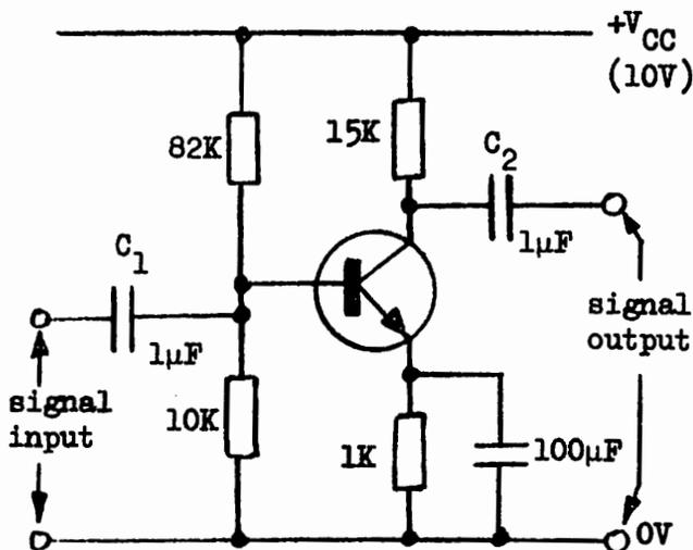
Fig. 3 : A practical transistor amplifier based on the circuit of Fig. 2
