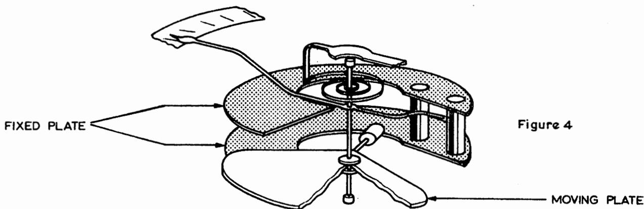
The attractive force is small and dependent on the voltage between the plates. Apart from the charging current, the meter takes no power from a d.c. source and very little from an a.c. source. It is therefore often used to measure high impedance, high voltage supplies as found in television receivers and monitors. The sense of the deflecting force is independent of
