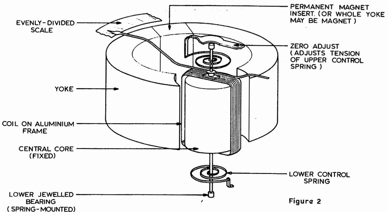
Moving coil meters usually have a uniform scale extending over a  $90^{\circ}$  arc. Due to the inertia of the moving parts, they indicate the average value of a varying current; they give no deflection for alternating currents above a few Hertz.
