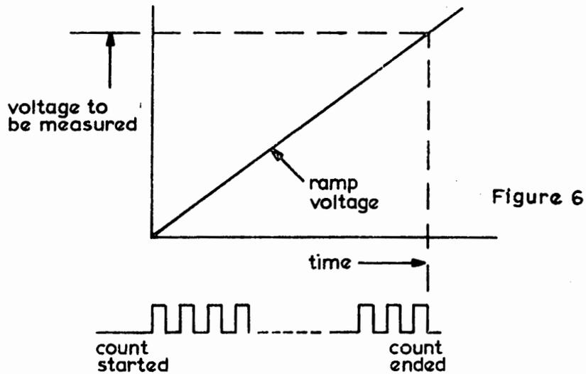
A ramp voltage is generated within the instrument which increases from zero to a maximum at a constant rate. A pulse generator is started at the same instant and is stopped when the ramp voltage is equal to the voltage being measured. The pulses are counted digitally and the total displayed using liquid crystal, l.e.d. or similar devices.
