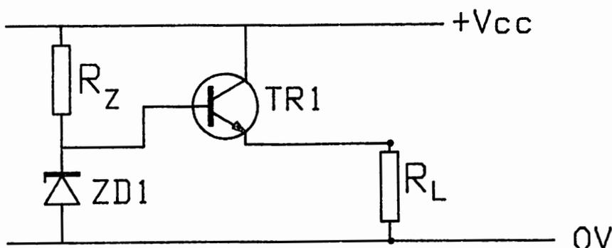
Fig. 9 P.S.U. Control Stage
