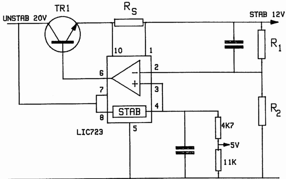
Fig. 15 An I.C. Voltage Regulator
