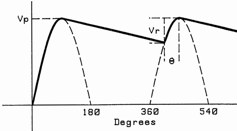
Fig. 3 Half-wave Smoothed Waveform
