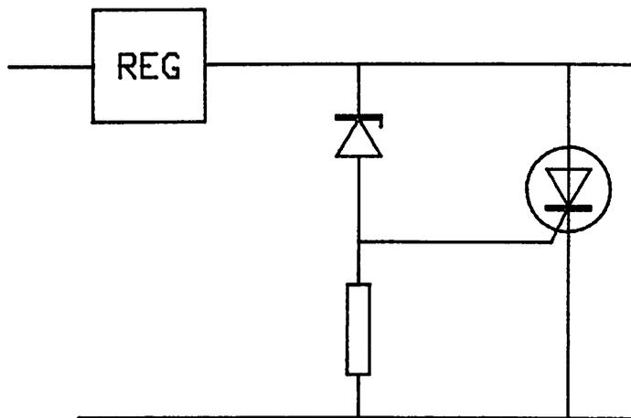
Fig. 13. Crowbar Overvoltage Protection
