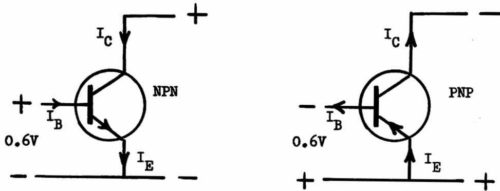
Figure 6 NPN and PNP Transistors
