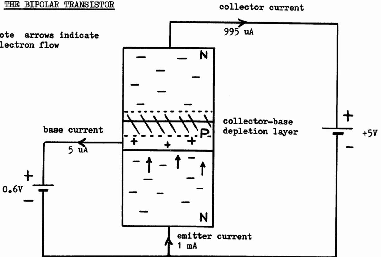
Figure 5 Bipolar Transistor Action
