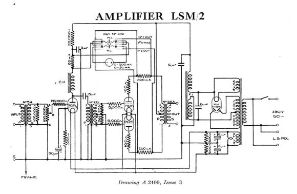
This is an A.C. mains-operated loudspeaker amplifier used in the loudspeaker units provided in the listening halls at London (Broadcasting House).
