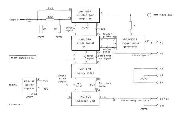
Fig. 1 Block Diagram of the AM18/519
