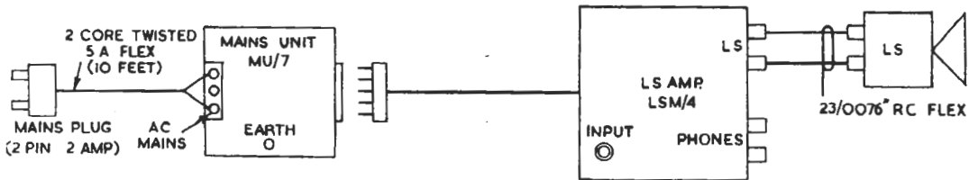
Fig. 13.7. LSU/1 Block Schematic
