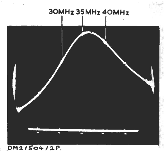
Fig. 2 Frequency Response of the DM2/504 as Measured at the Output of the Receiver 1
