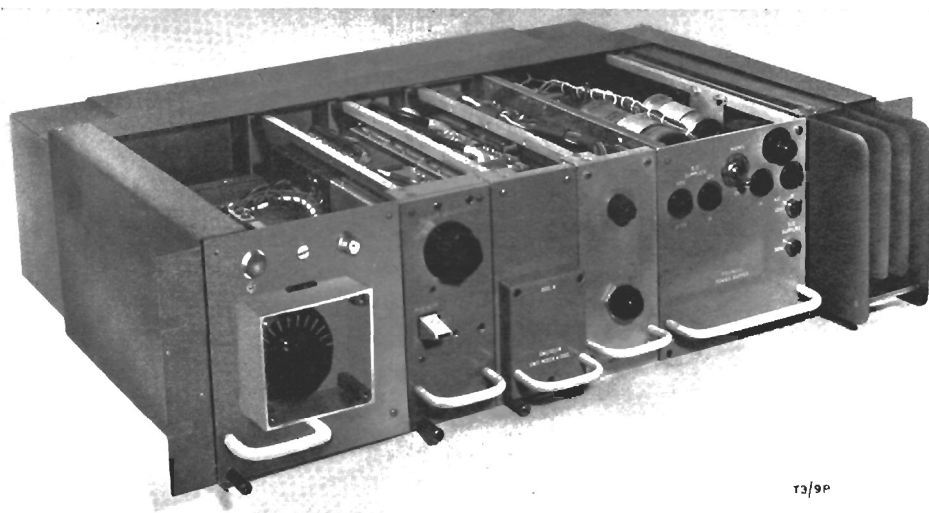
Fig. 3.1. EP7/4 and EP7/4A Drives: Typical Assembly
