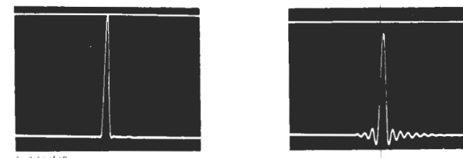
Fig. 5 1T-pulse Response: (a) output of generator (b) output of filter
