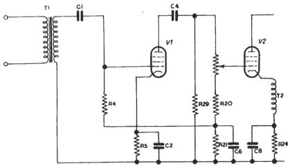
Fig. 8.2. Circuit for 80-dBgain
