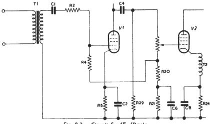
Fig. 8.3. Circuit for 65-dBgain
