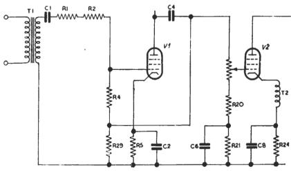
Fig. 8.4. Circuit for 50-dBgain
