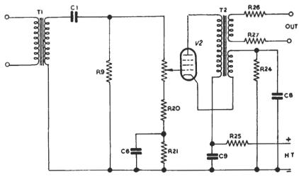
Fig. 8.5. Circuit for 35-dB gain
