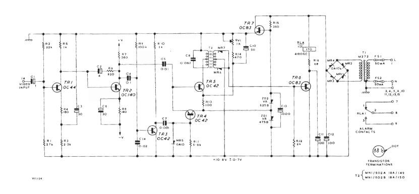
Fig. 2.1. Circuit of the MN1/502A and MN1/502B
