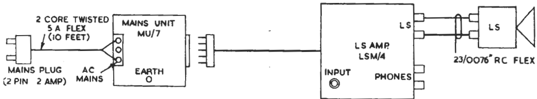
Fig. 13.7. LSU/1 Block Schematic
