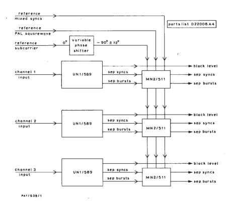
Fig. 1 Block Diagram of the PA1/538 Showing Pulse and Video Circuits
