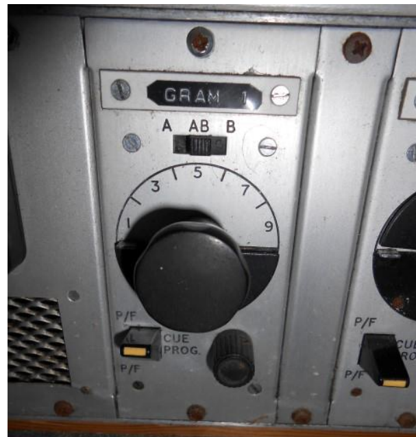
Figure 2. One of the preamp modules. Note that each module is labelled: this one is GRAM 1
