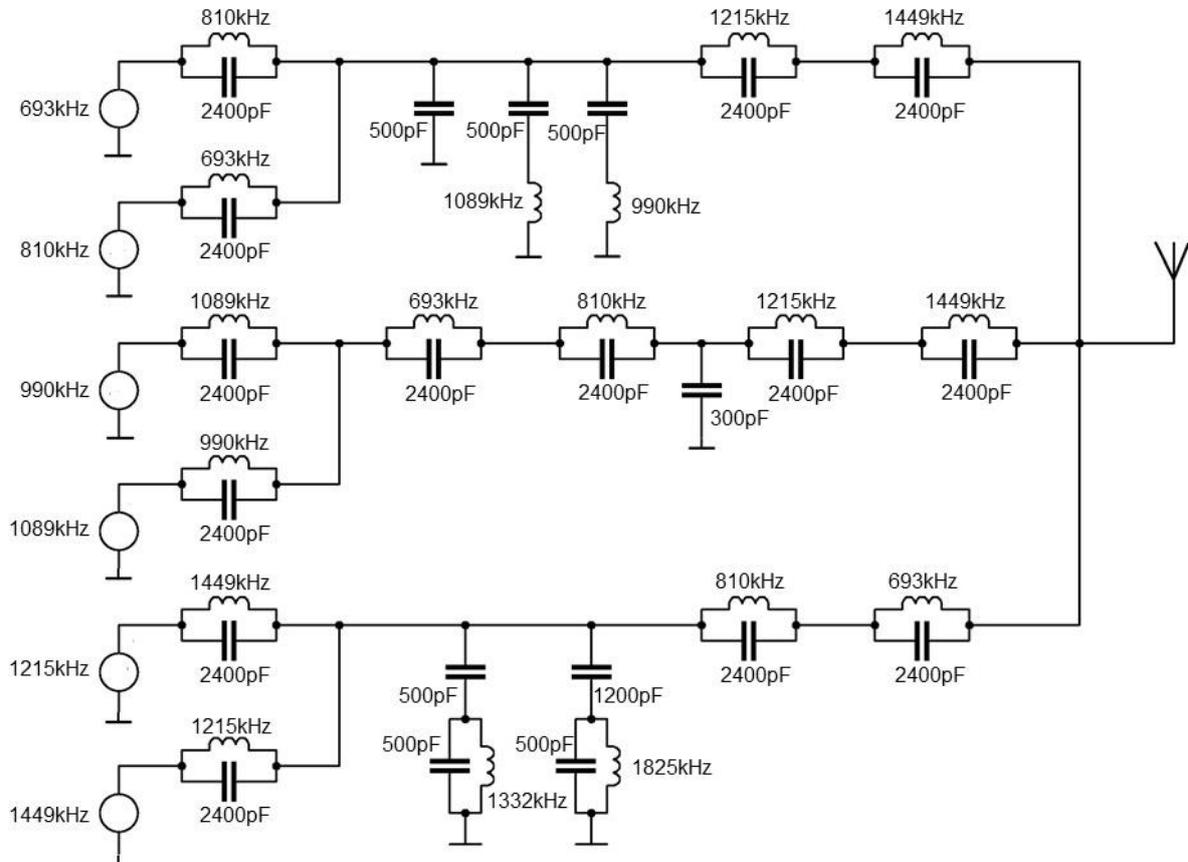
Figure 2. Circuit diagram of the duplexer at Redmoss
