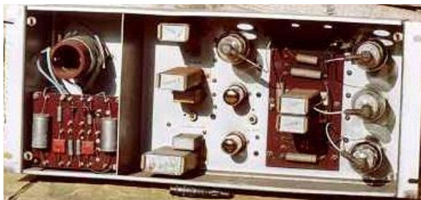
Figure 4. The drive regulator chassis containing two 6AG7s and four 807s
