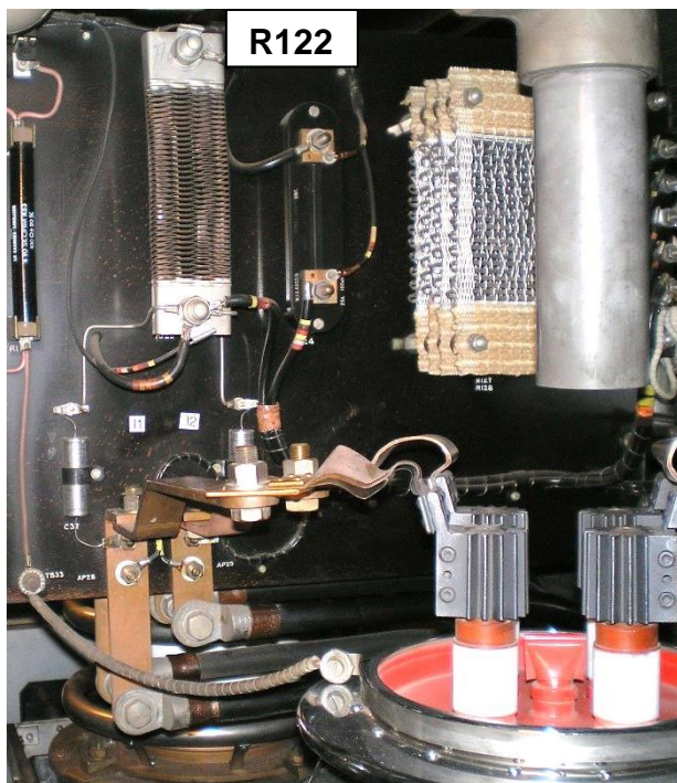
Figure 1. A typical high-wattage, low-value current-sensing resistor. It is the expanded metal element labelled as R122
