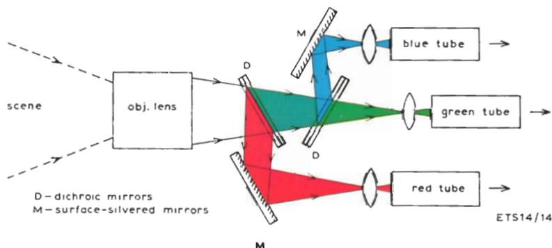
Fig. 4.2 Arrangement of dichroic mirrors in a colour television camera
