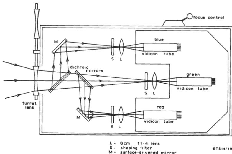
Fig. 4.8 Optical system of E.M.I. colour television camera
