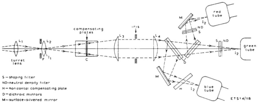
*Fig. 4.6 Optical system of R.C.A. colour television camera*
