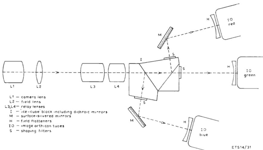
Fig. 4.7 Prism-block optical system for colour television camera
