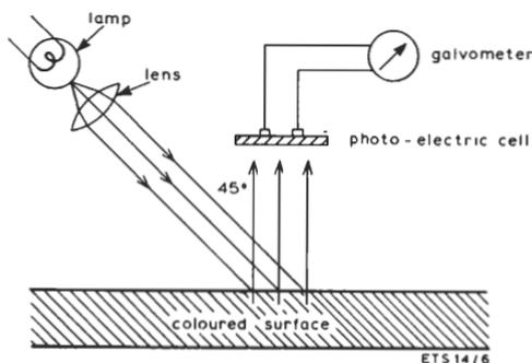
*Fig. 2.5 Determination of the spectral reflection characteristic of a coloured surface*
