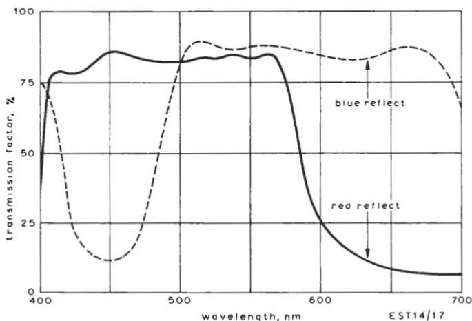
Fig. 4.5 Transmission characteristics of dichroic mirrors
