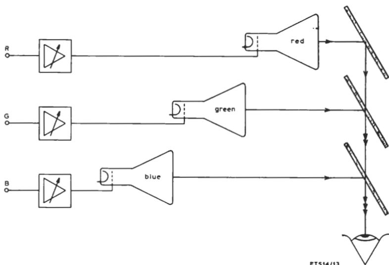
Fig. 4.1 Production of a colour picture by use of three cathode ray tubes
