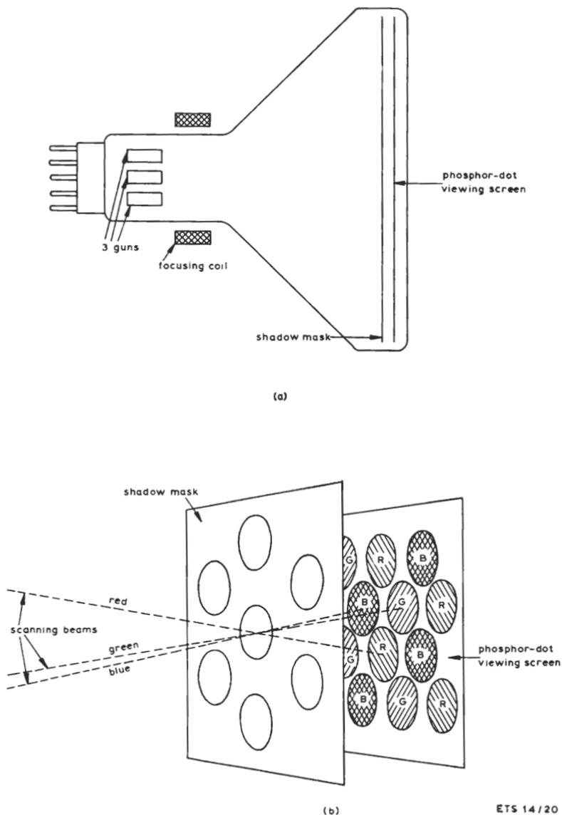
Fig. 4.9 R.C.A. shadow-mask picture tube (a) with details of the mask and phosphor dot screen (b)
