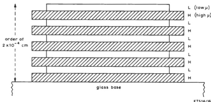
Fig. 4.4 Construction of a dichroic mirror
